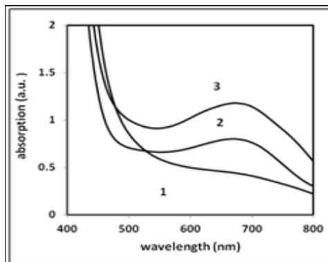
Figure 3(b): UV-Vis absorption spectra of alcoholic extract of "Mesua ferrea" at (1)  $25^\circ C$ , (2),  $50^\circ C$  and (3)  $100^\circ C$
