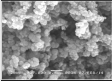
Figure 2 (a) SEM images of  $TiO_2$  nanoparticle
