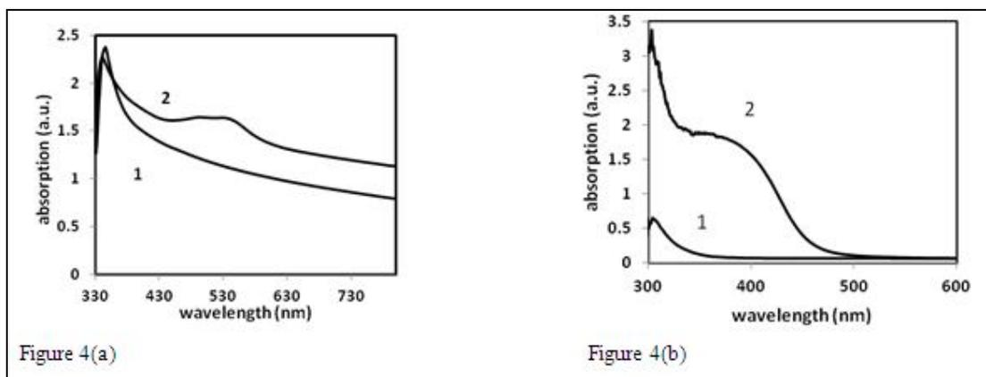
Figure 4: (a)-4(b) show the comparison of UV-Vis absorption spectra of the TiO<sub>2</sub> thin film (1) and dye loaded (2)TiO<sub>2</sub> thin film (soaked with dye A and B respectively ).
