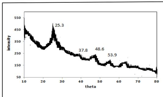
Figure 1(b): X-ray diffraction pattern for TiO<sub>2</sub>
