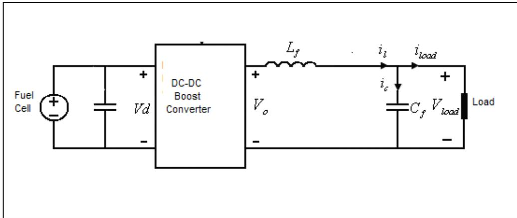
Figure 4: Shows the fuel cell connected dc-dc boost converter with L-C filter
