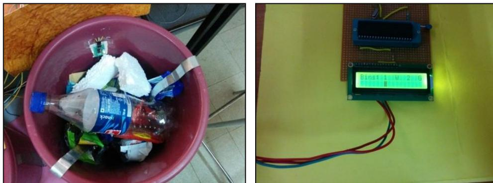
Figure 8: Bin 1 is filled by level sensor and display is shown on LCD
