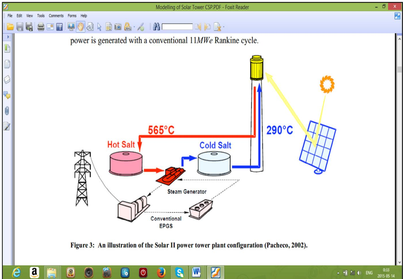
Figure 2: Simplified schematic of a solar power tower system using molten salt thermal storage.
