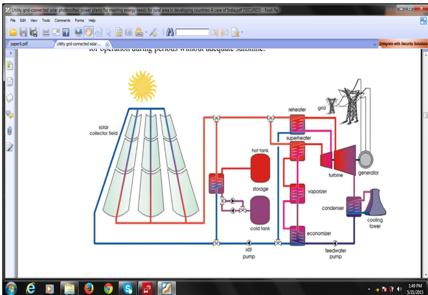
Figure 3: Simplified schematic of a parabolic trough system
