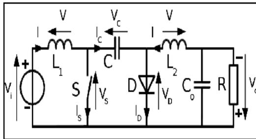
Figure 4: circuit diagram of a Boost-Buck converter
