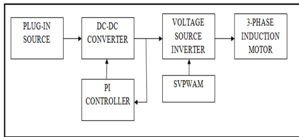
Figure 1: basic block diagram for conventional method
