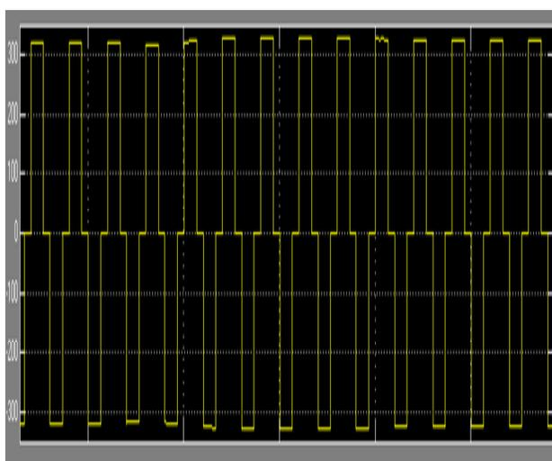
Figure 6: output voltage of VSI inverter
