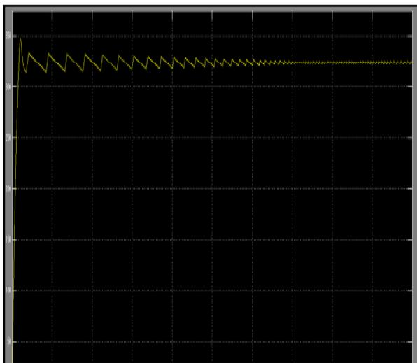
Figure 11: Cuk Converter output
