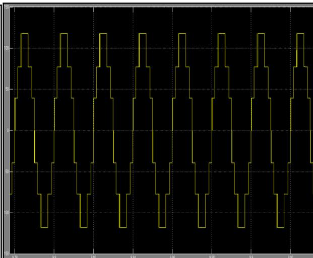
Figure 9: output Voltage of Sevenlevel Inverter
