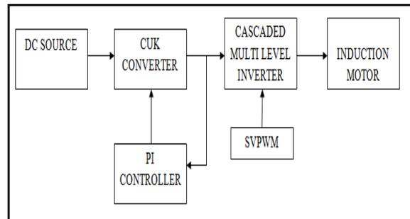
Figure 2: basic block diagram for proposed method
