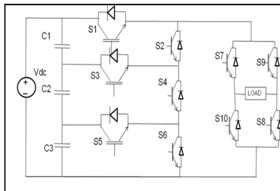
Figure 3: Cascaded Multilevel Inverter
