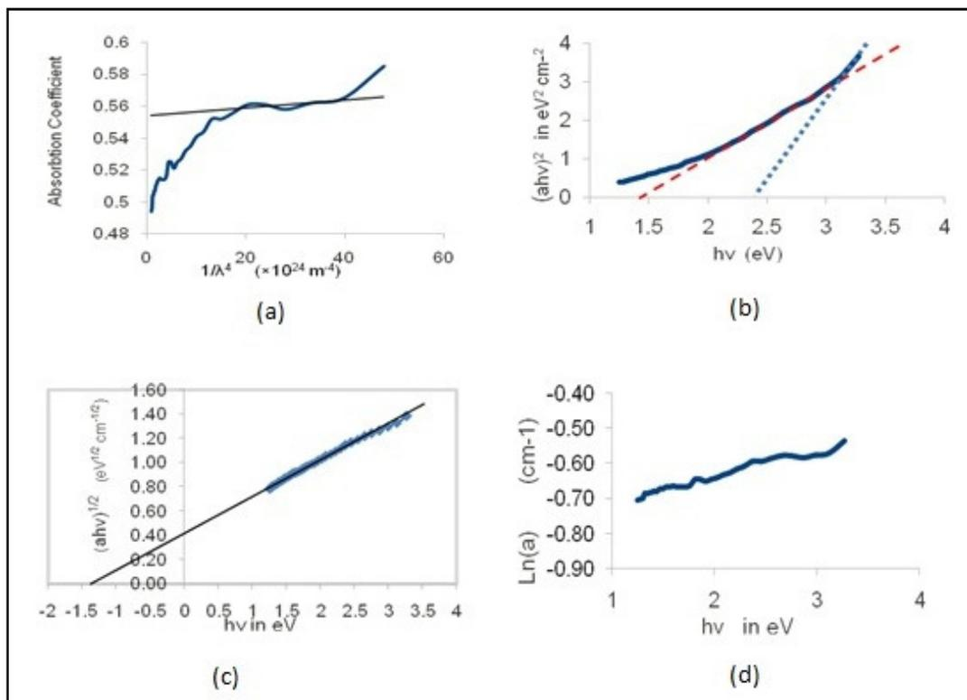
Figure 4: Absorption coefficient against  $1/\lambda^4$  (b) shows  $(ah\nu)^2$  against photon energy (c) shows  $(ah\nu)^{1/2}$  against photon energy (d) shows  $\text{Ln}(a)$  against photon energy.
