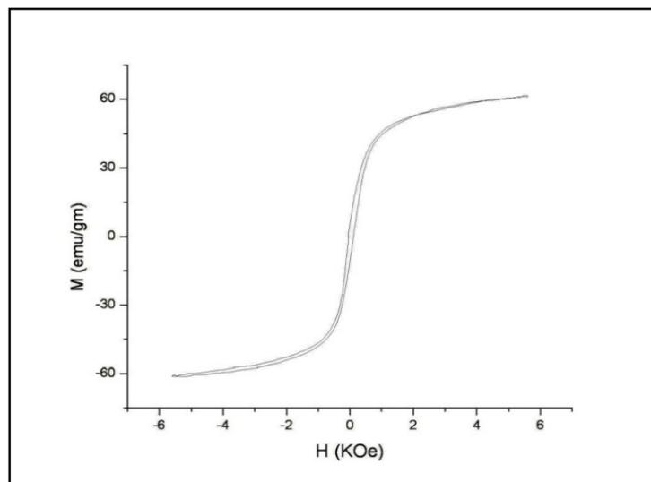
Figure 2: Hysteresis of the IOUP at room temperature
