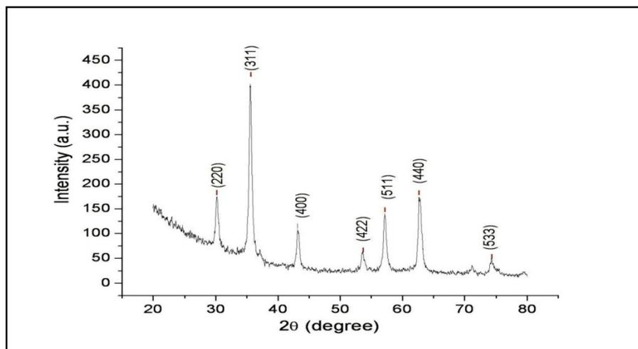
Figure 1: X ray diffraction of IOUP
