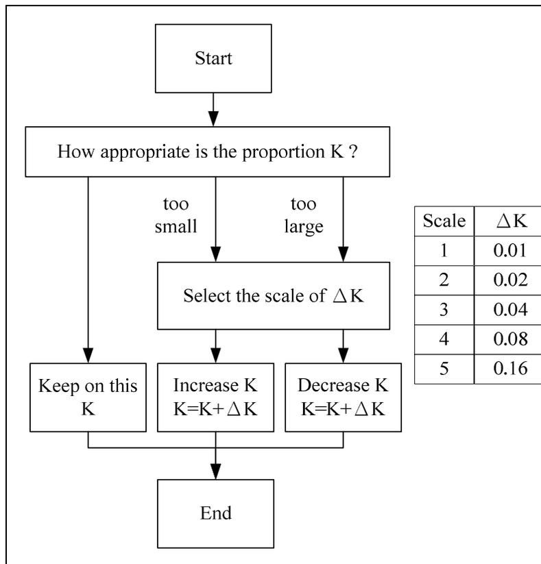
Figure 2: System identification and parameter controller flow chart.
