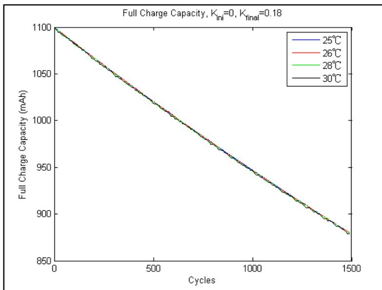
Figure 3: The FCC of cells cycled at different temperatures with adaptive control versus cycles.
