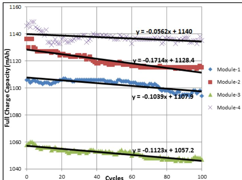
Figure 8: The capacity of modules without control versus cycles.
