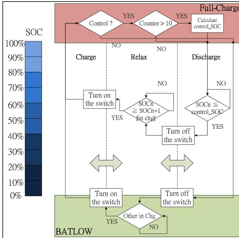
Figure 7: The switches control flow chart.
