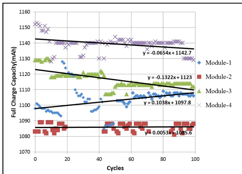
Figure 9: The capacity of modules using adaptive control versus cycles.
