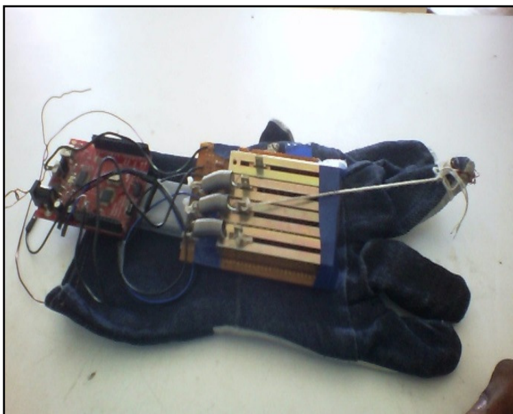
Figure 12: Hardware structure of sensing gloves
