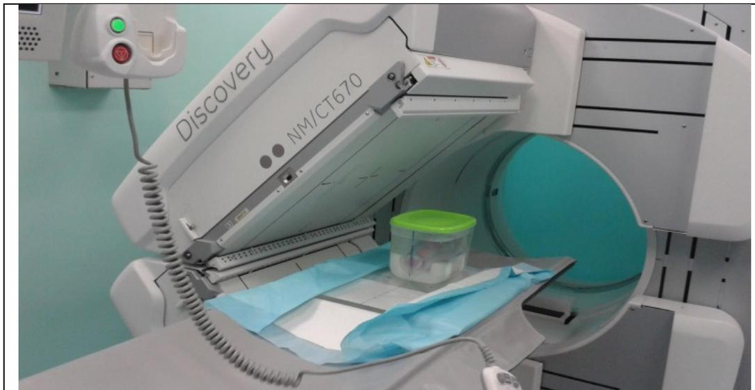
Figure 3: Phantom positioned at the center of the table while acquiring SPECT images
