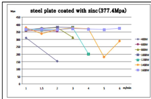
Figure 5: Results of UTM test in butt joints (steel platecoated with zinc)
