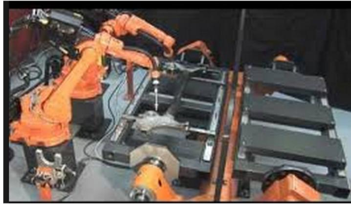
Figure 1: The robot-based remote laser welding system
