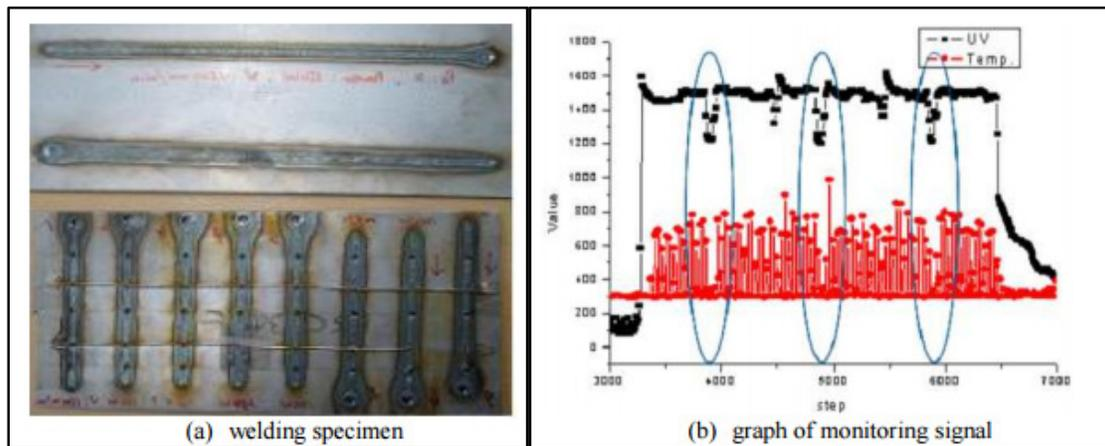
Figure 4: The results of plasma intensity detection using an Nd:YAG laser
