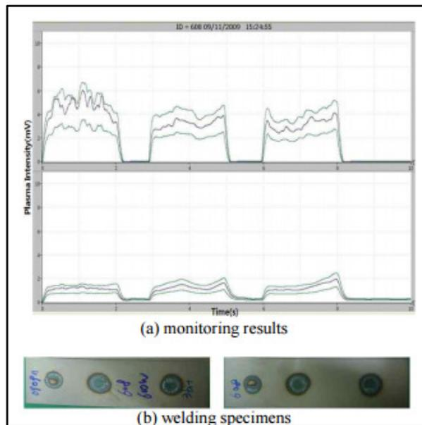
Figure 7: Results of quality monitoring during remote laser welding for three circle patterns
